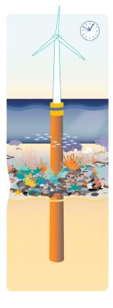
Figure 3: a schematic representation of life span extension of the wind turbine and the reuse of its foundation. The foundation is designed (overengineered) in such a way that it is suitable for a larger, modern turbine.
