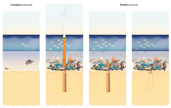
Figure 2: complete or partial removal of offhore wind turbines
